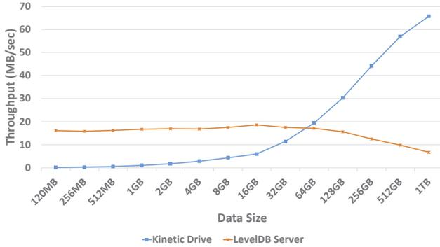
Figure 2: Comparison of Write throughput between Kinetic Drive and LevelDB server [17]
