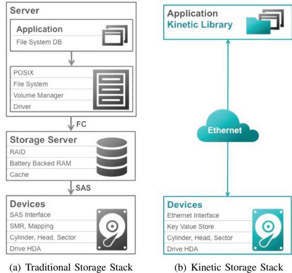
Figure 1: Comparison of Traditional and Kinetic Storage Stack [14]
